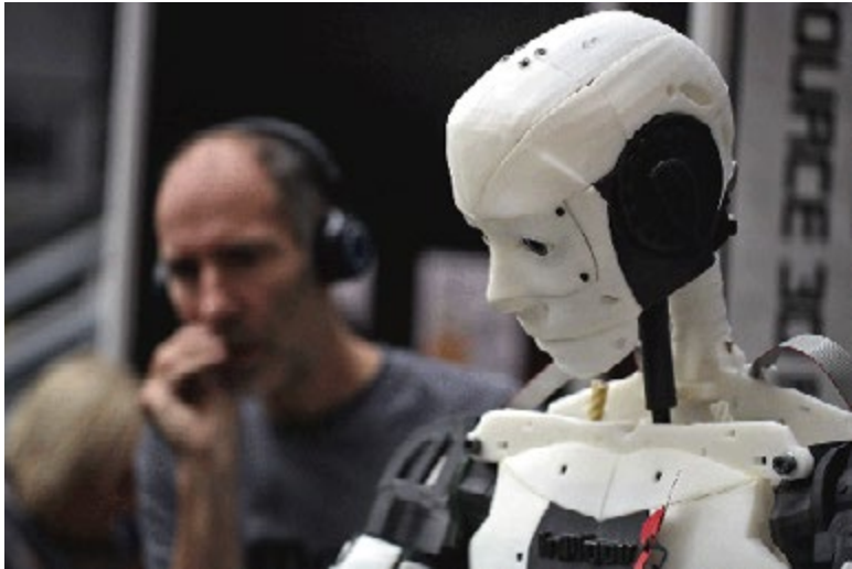
InMoov animatronic android robot, made from 3-D printed parts.
