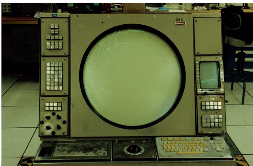
World-War II era Air Traffic Control Console, in use into 1990s. The United States' Air Traffic Control system shared many of the characteristics of the SAGE air-defense system. Because of the large initial investment made by the United States in these systems, they remained in use even though they were technically obsolete. This round radar screen, derived from a World War II era defense system, was being used for U.S. commercial air traffic control into the 1990s. Smithsonian Institution.
