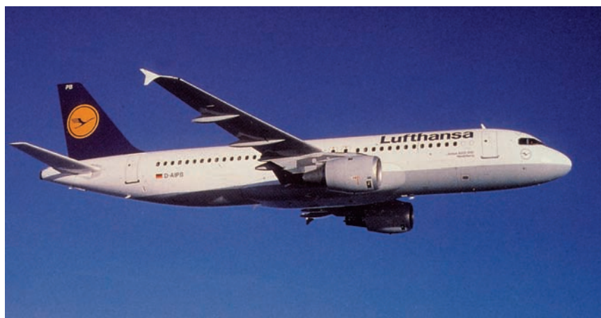
Airbus A-320. The computer controls developed to land the Lunar Module were transferred to commercial aircraft. The Airbus A-320, which entered service in the mid-1980s, was the first to adopt this—fly-by-wire—technology. It is now standard on nearly all commercial jets. Lufthansa.
