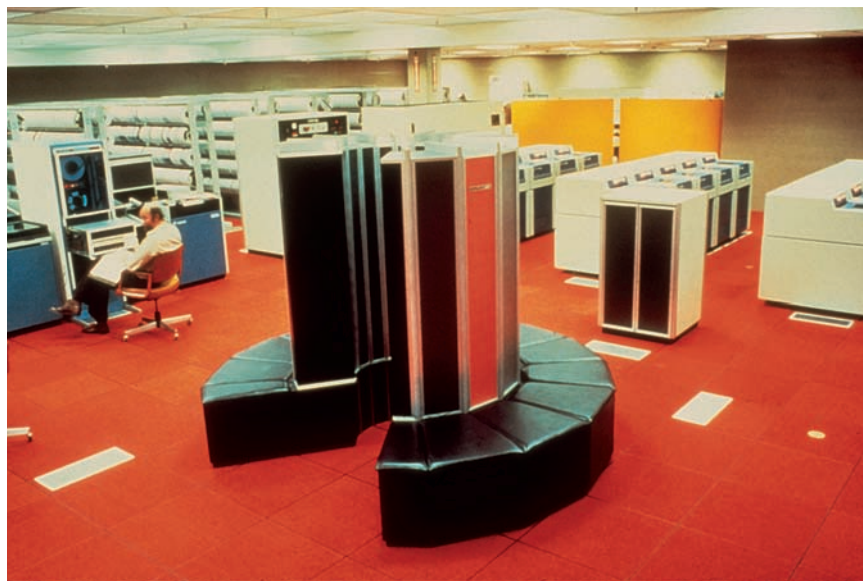
CRAY-1 Supercomputer, ca. 1976. The CRAY-1, designed by Seymour Cray, was the first "supercomputer," which could compete with wind tunnels in analyzing air and spacecraft design. CRAY Research, Inc.
