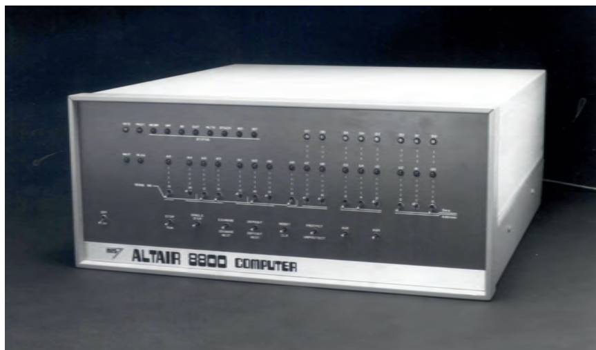
Altair Personal Computer, 1974. A small hobbyist company, MITS, of Albuquerque, New Mexico, introduced this computer as a kit in 1974, and it sparked the revolution in personal computing. Smithsonian Institution.
