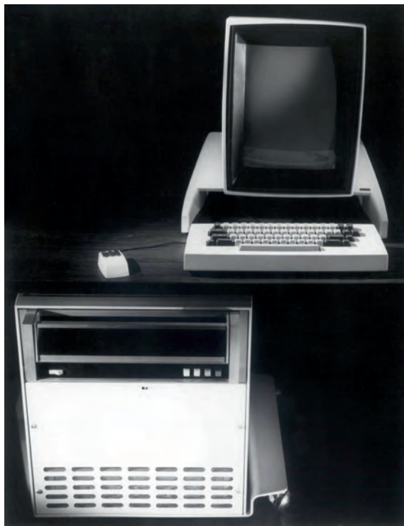
Xerox "Alto" Workstation, ca. 1973. The Alto was designed and built at the Xerox Palo Alto Research Center (PARC) in California. It pioneered in the use of a mouse and a graphical user interface, which eventually became common in personal computers. Altos were linked to one another by Ethernet and sent their output to laser printers, both Xerox innovations. Smithsonian Institution.
