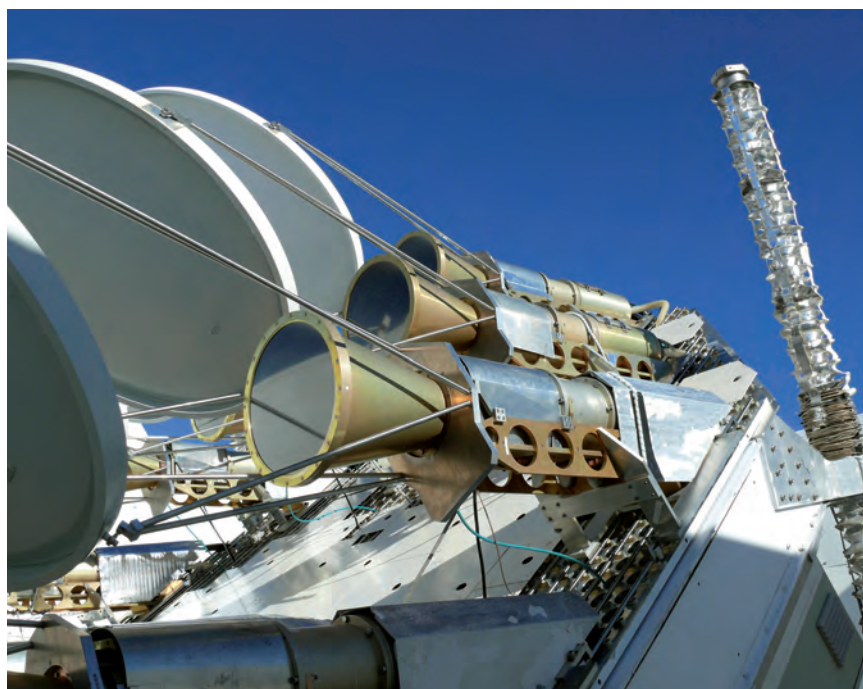
Figure 3. The Very Small Array, which belongs to the IAC and the Universities of Cambridge and Manchester, is one of the instruments installed at the Canary Islands' Astrophysical Institute's Teide Observatory for measuring anisotropies in the Cosmic Microwave Background. The observatory has been systematically measuring this primeval radiation with different instruments and techniques for over twenty years. IAC.
