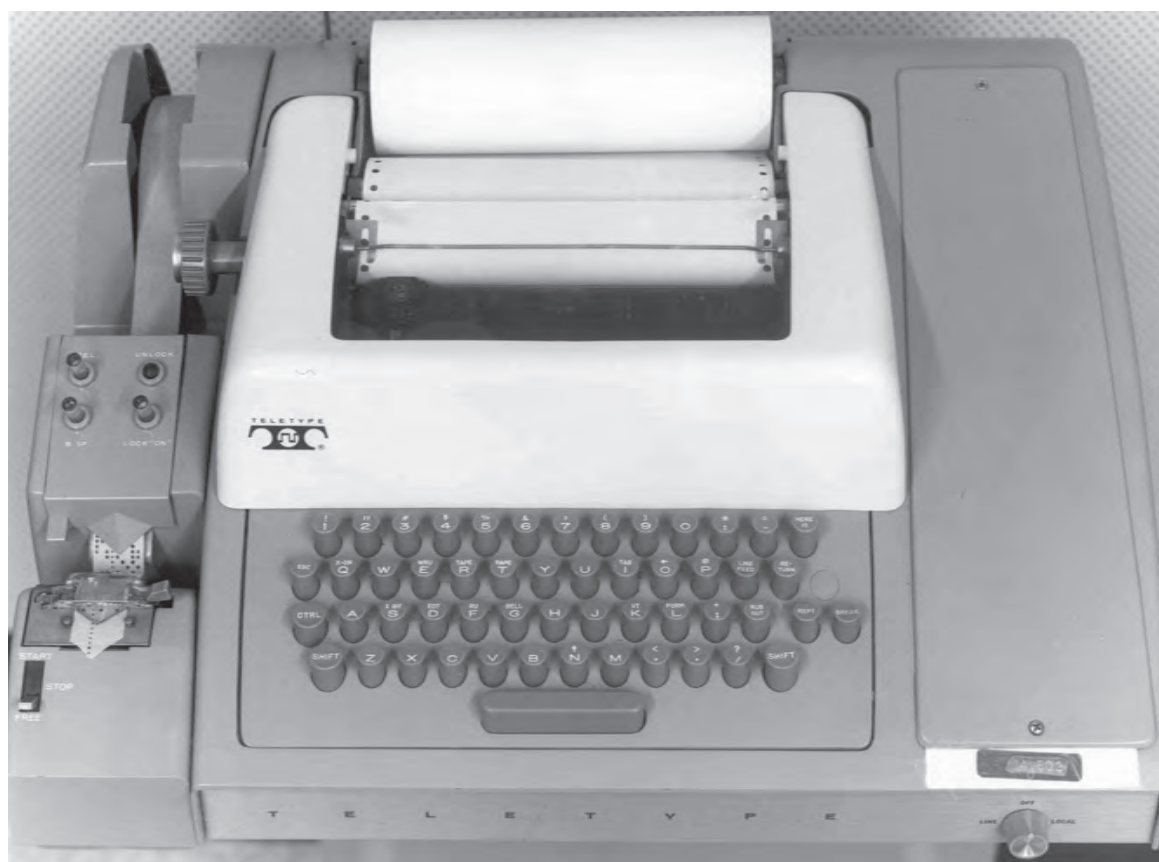
Teletype Model ASR-33. The ARPANET used this modified Teletype as a terminal. Note the "@" sign, which was adopted for e-mail and has become the icon of the networked age. Smithsonian Institution.
